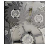
Feeder wheels grab the seed from the disk and deposit it onto a flighted belt.
